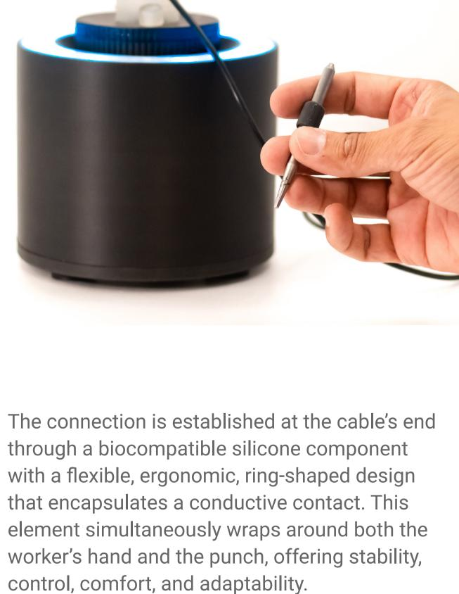
different sizes to fit various punch tools. The punch tool is inserted into this component and positioned at a precise distance from the charged diamond powder, ensuring that the correct amount of particles adheres to the tool to form a precise marking. The punch tool is electrically grounded through a flexible cable connected
