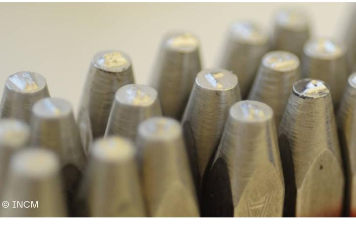
The assay offices in Portugal partnered with a research centre on human-centred digital technology to develop an innovative solution that could create unique and unclonable marks on metal artefacts to certify their authenticity, using a stamping process (punch marking) similar to that traditionally used for hallmarking precious metals.
