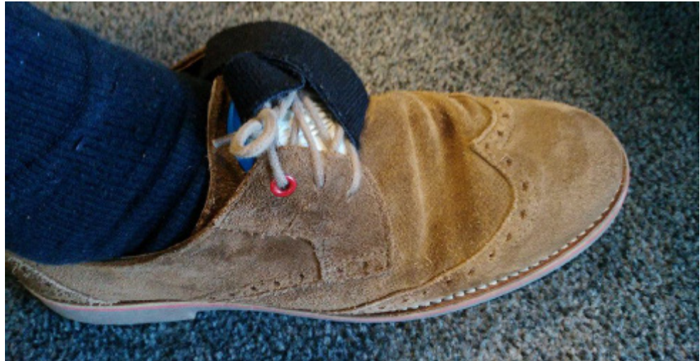
Fig2. Placement of the IMU on the foot – under the shoelaces.
